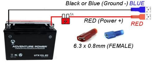
FLEXIBLE CABLE - 2x1.5mm<sup>3</sup> (square millimeter)
